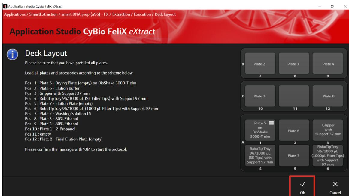
Figure 17: Deck layout for checking the correct positions of all plates and accessories.
