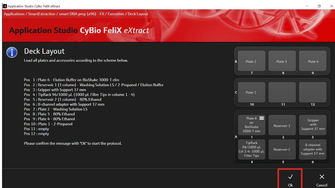
Figure 8: Deck layout for final hardware check for the prefilling.
