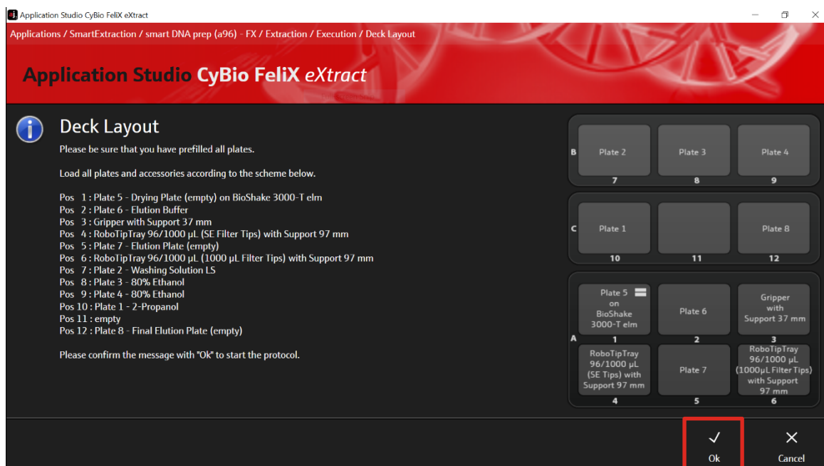
Figure 17: Deck layout for checking the correct positions of all plates and accessories.
