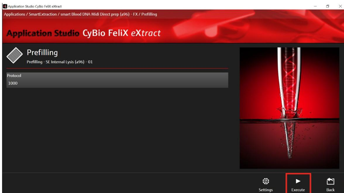
Figure 26: Selection of the prefilling protocol for up to 1000  $\mu\text{L}$  sample volume.
