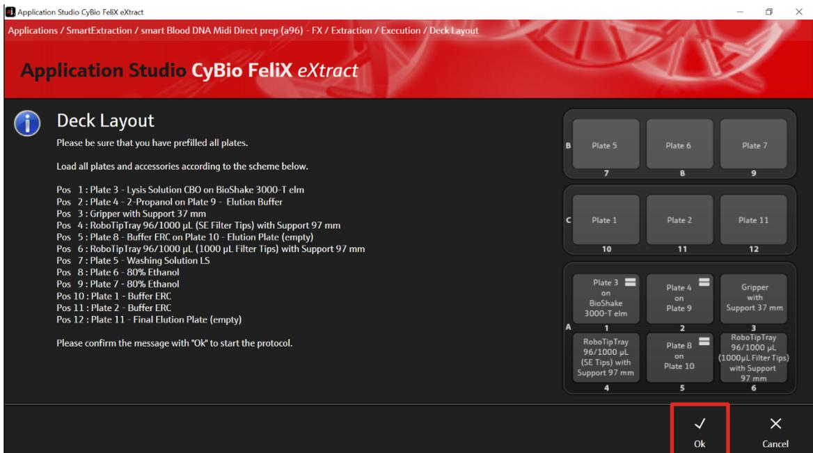
Figure 36: Deck layout for checking the correct positions of all plates and accessories.
