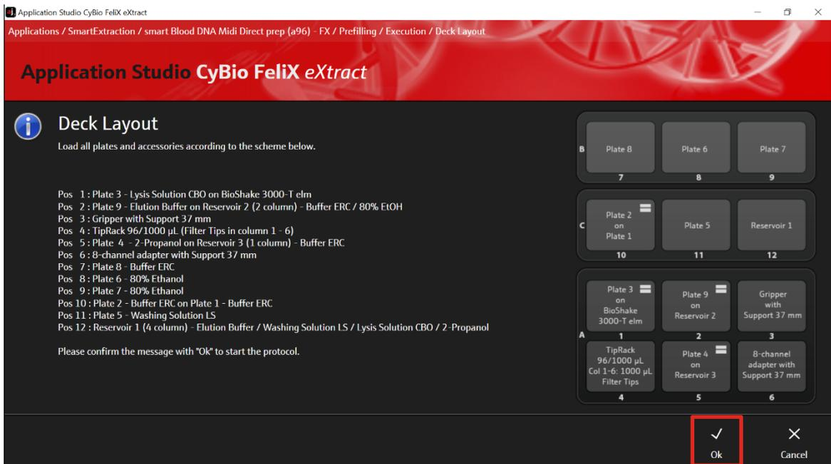
Figure 27: Deck layout for checking the right positions of all plates and accessories.
