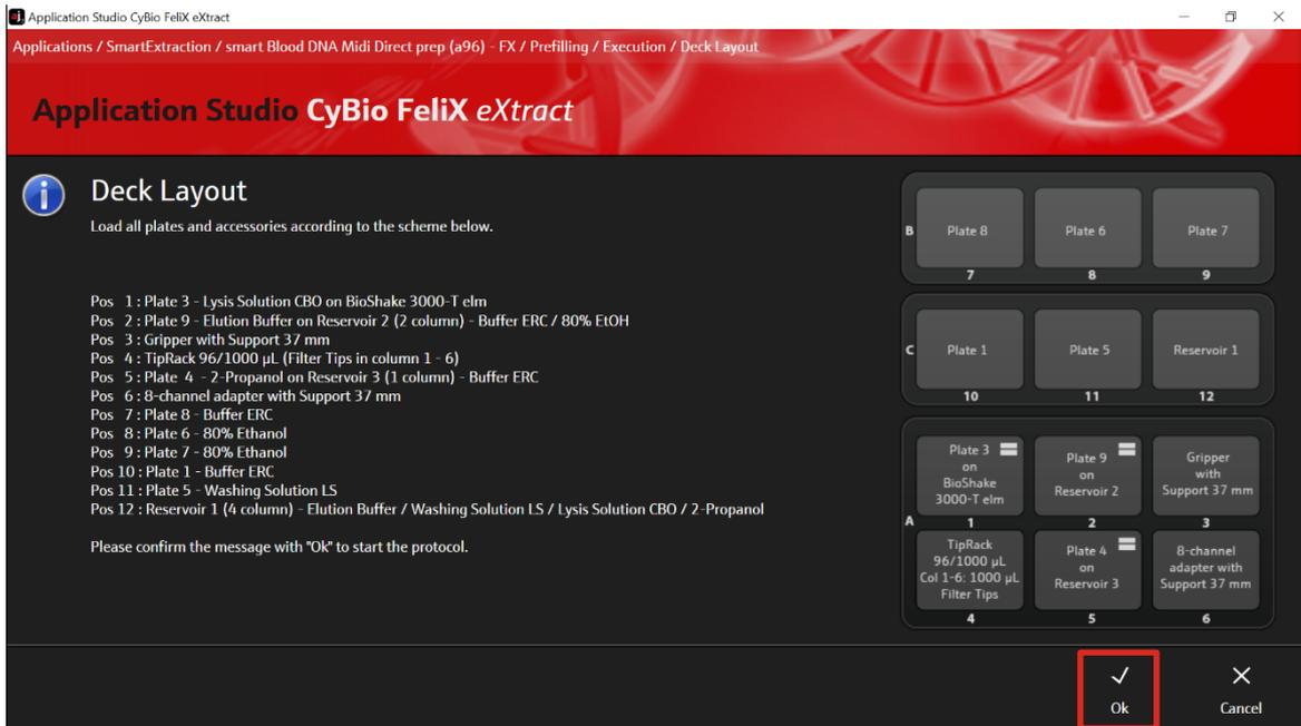
Figure 9: Deck layout for final hardware check for the prefilling.
