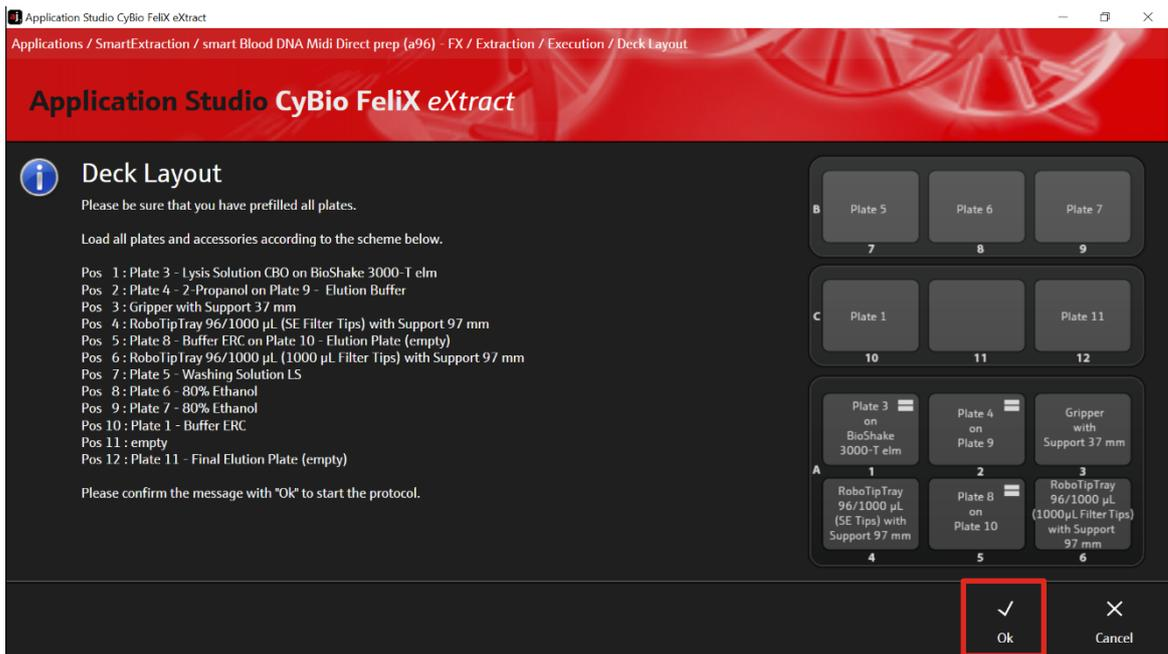
Figure 18: List of deck positions and corresponding plates.
