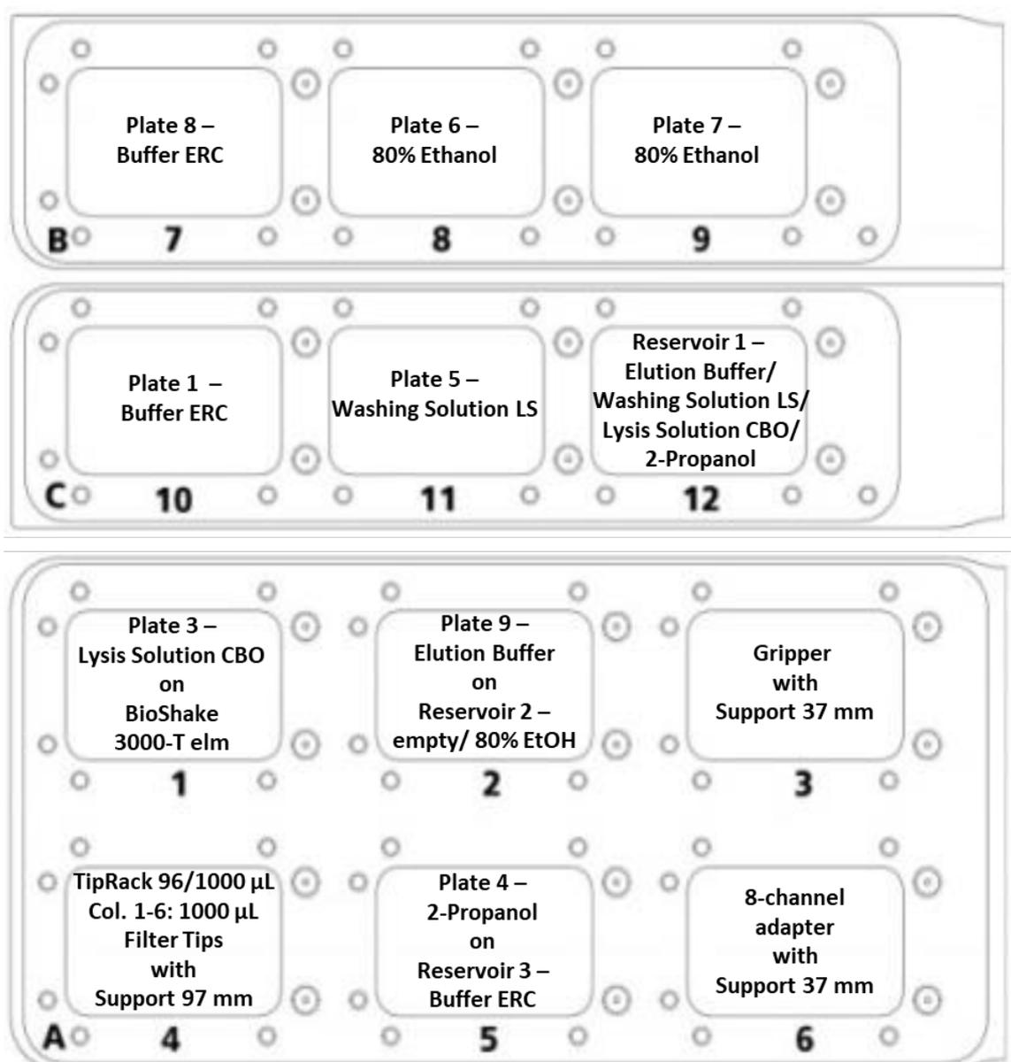
Figure 3: Deck Layout for the prefilling protocol for up to 500  $\mu$ L sample volume.
