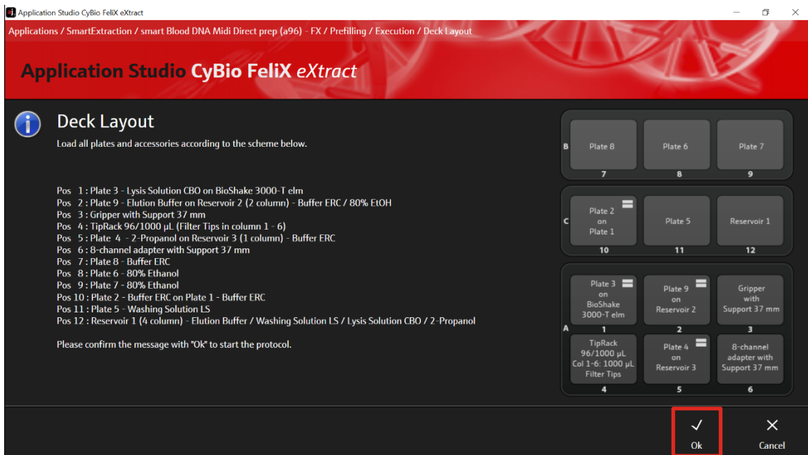
Figure 27: Deck layout for checking the right positions of all plates and accessories.
