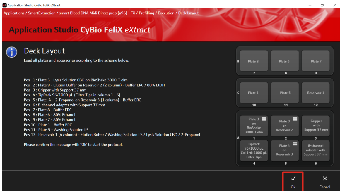
Figure 9: Deck layout for final hardware check for the prefilling.
