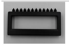
Reagent Plates / Reagent Strips are prefilled with extraction reagents and are sealed with a foil. Prior to use this foil has to be pierced manually, by using the piercing tool.
