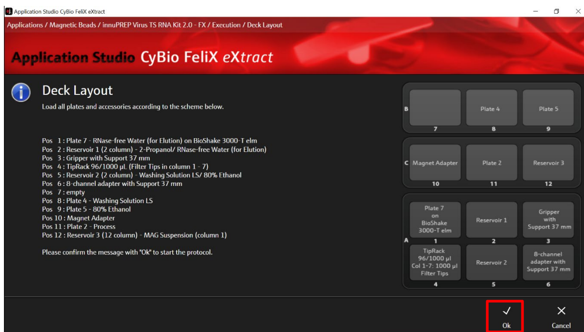
Figure 8: Deck layout for the final hardware check of the prefilling.
