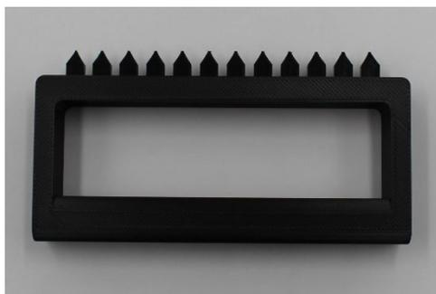
Reagent Plates or Strips are prefilled with extraction reagents and are sealed with a foil. This foil has to be pierced manually before use, by using the piercing tools (12 well piercer).
