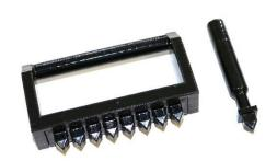
Reagent Plates or Strips are prefilled with extraction reagents and are sealed with a foil. This foil has to be pierced manually before use, by using the piercing tools (Single well piercer or 8 well piercer).
