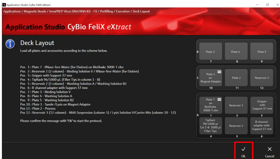
Figure 25: Deck layout for checking the correct positions of all plates and accessories.
