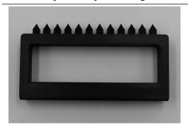
Reagent Plates or Strips are prefilled with extraction reagents and are sealed with a foil. Prior to use this foil has to be pierced manually, by using the piercing tools (12 well piercer).
