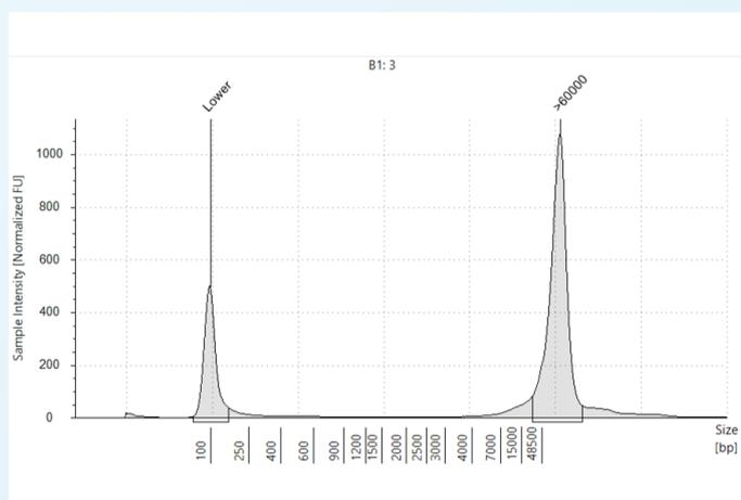
To determine the DNA quality, 1 µl DNA of sample 3 was used on Agilent 4150 TapeStation System (Agilent, gDNA Assay) The results indicate that majority of the DNA is longer than 60,000 bp and shows a high integrity. The DNA yield is very high and the ratios between 260/280 and 260/230 are excellent.
