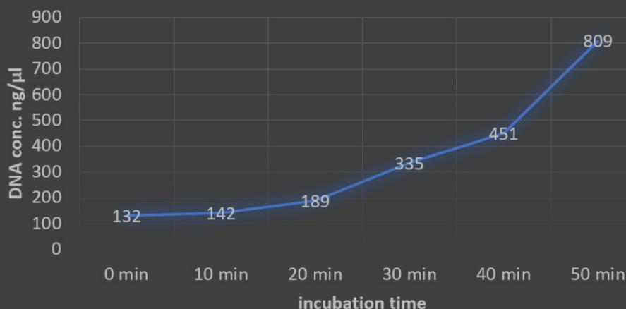
Sample: 132 ng/µl lambda DNA in 200µl where concentrated with addition of TCT Beads to the sample and continuously measurement of DNA concentration (UV-Vis).
